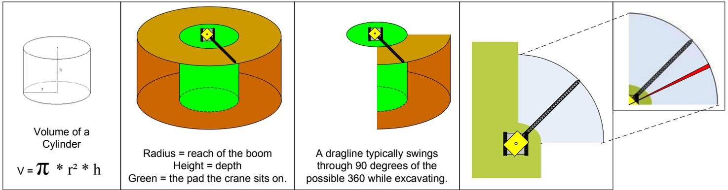
The images above are provided to give you a visual reference showing an area of material which a dragline crane can reach from a given position. Typically a dragline will follow a cut line and rotate out to a maximum of 90 degrees. This area of reach is represented in the third, fourth, and fifth images. In the last image, a red wedge is visible.
